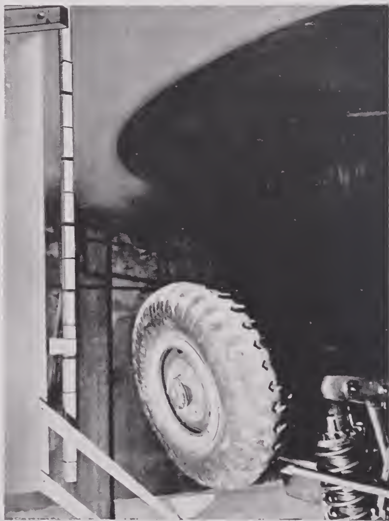
FIGURE 24. Experimental wheel unit clearing height of 19 inches.
